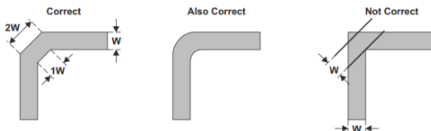
Figure 15 Appropriate Signal Wiring Leads
